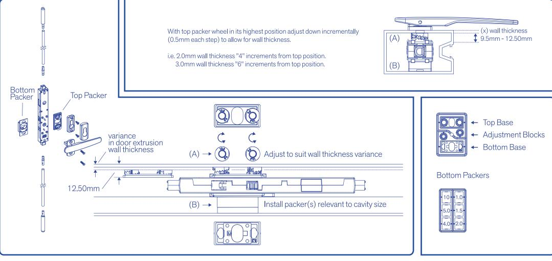
The Top Packer (A) is required to suit the various door extrusion wall thickness. These rotary wheels incorporate incremental adjustment of 0.5mm. Correct adjustment of the wheels result in the cylinder housing being held securely and the screws achieving the correct purchase depth into the lockbody.
