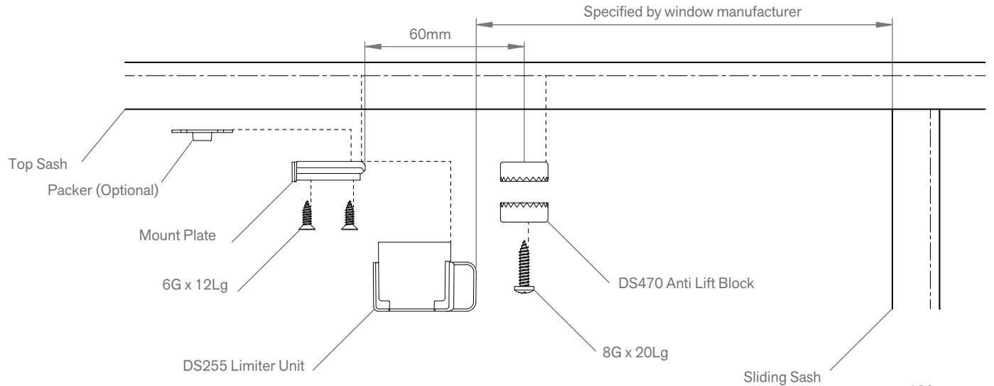
**1.** Use the *mount plate* to mark two centre holes at the distance specified by the window manufacturer from the sliding sash.
