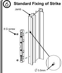
Using the machining details, machine holes for strike on jamb. For standard fixing, the holes must be Dia.3.5mm. Screw in place with 2 x 8G screws, but do not tighten.
