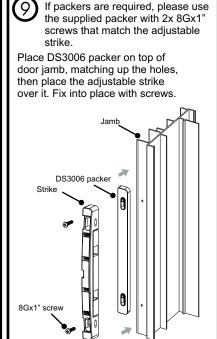
Once the strike is on the door jamb, test to see tongues engage the strike. If the tongues do not engage, adjust the vertical and horizontal adjustments. Keep the strike and lock parallel. Vertical
