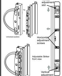
Once the lock is working correctly, place cover over strike using the 6G screw supplied. 6G screw Cover
