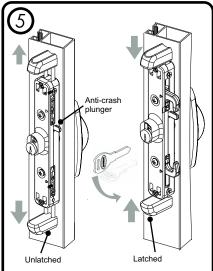
Check function of lock by using the key internally & externally then manually activating the levers. Tongues should move freely. NB. Make sure to depress the anti-crash plunger to activate the tongues & levers.
