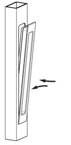
Angle the flush pull and lower the side with the wedge into the cutout.
