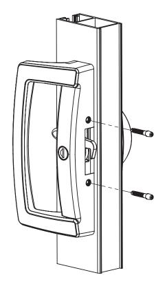
**8.** With the handle assembly complete, cycle test the lever and both interior & exterior cylinders to ensure they function correctly including inserting, operating and removing key.
