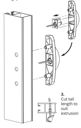
**3.** Place lock on inside of stile, aligning the centre holes for exterior cylinder tail to locate into interior cam. Fasten with 2 x M5 screws.
