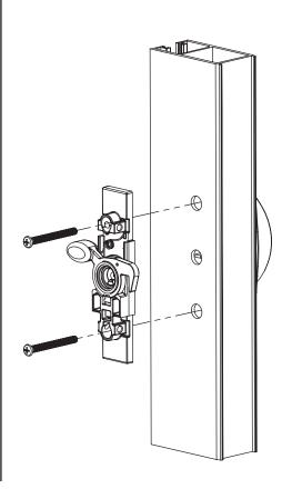
**4.** Ensure by cycling the external cylinder with key, that the internal lever operates smoothly.
